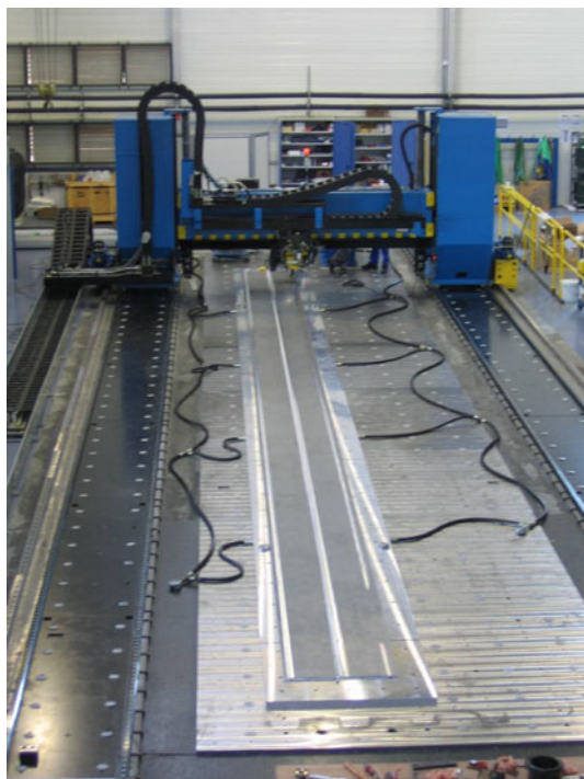
Fig. 6 Friction stir welded 17-m long panel in 2050 alloy. Trials were performed at the Institut de Soudure, Metz, France
